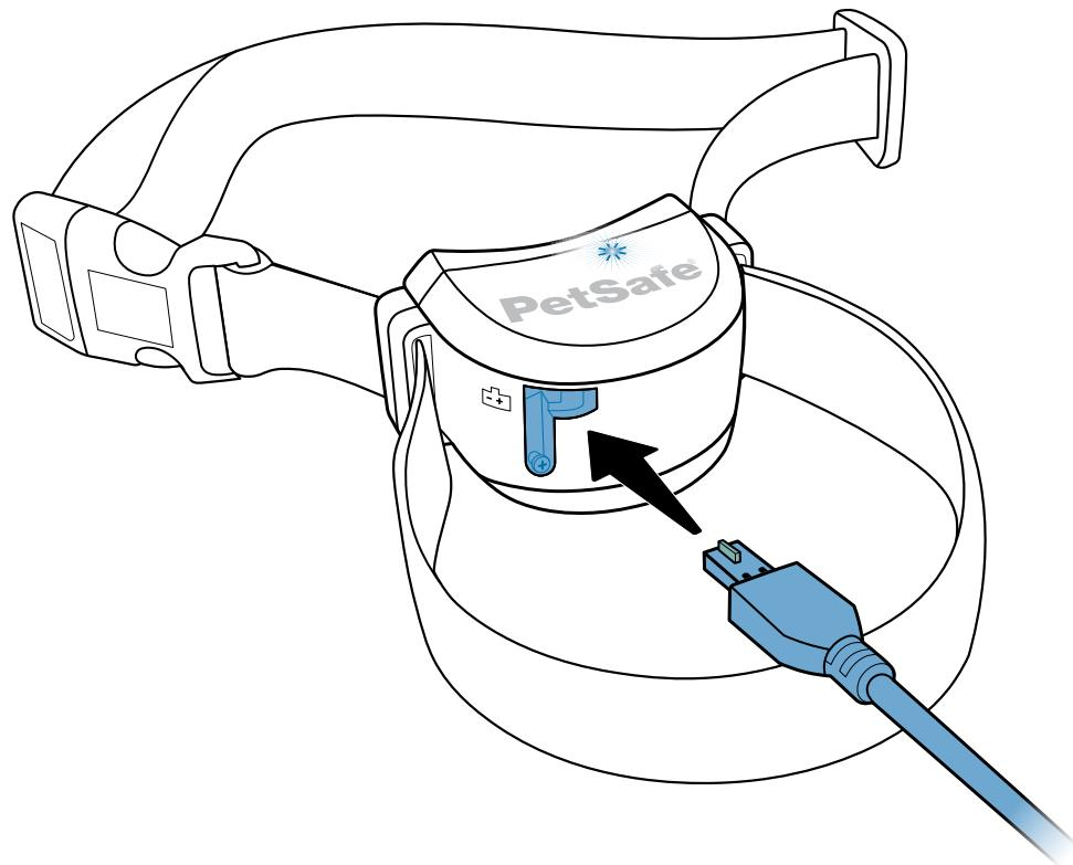
**EN** To start, you will need to locate the charging jack on the front of the collar. This is under the strap, covered by a rubber plug.
