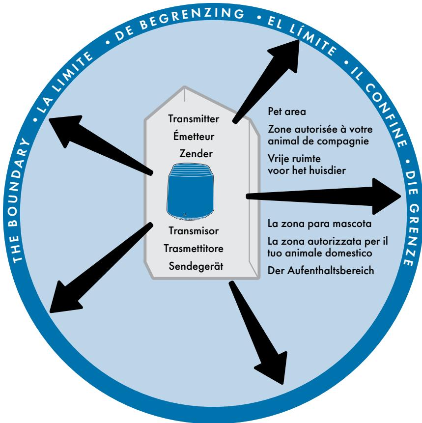
**EN** Make sure the transmitter is at least 70 cm above the floor on the ground level of your home in a dry, well ventilated area where temperatures do not go below -10 °C or above 40 °C.
